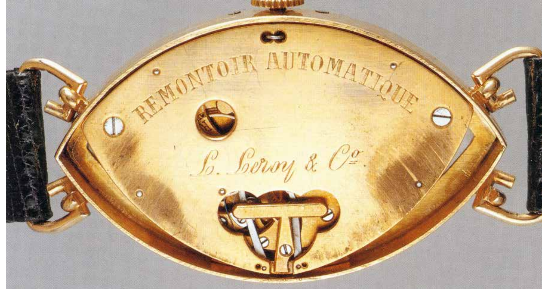
Leroy, automatic watch, movement, 1922 ◦ Leroy, Automatikubr, Werk, 1922
